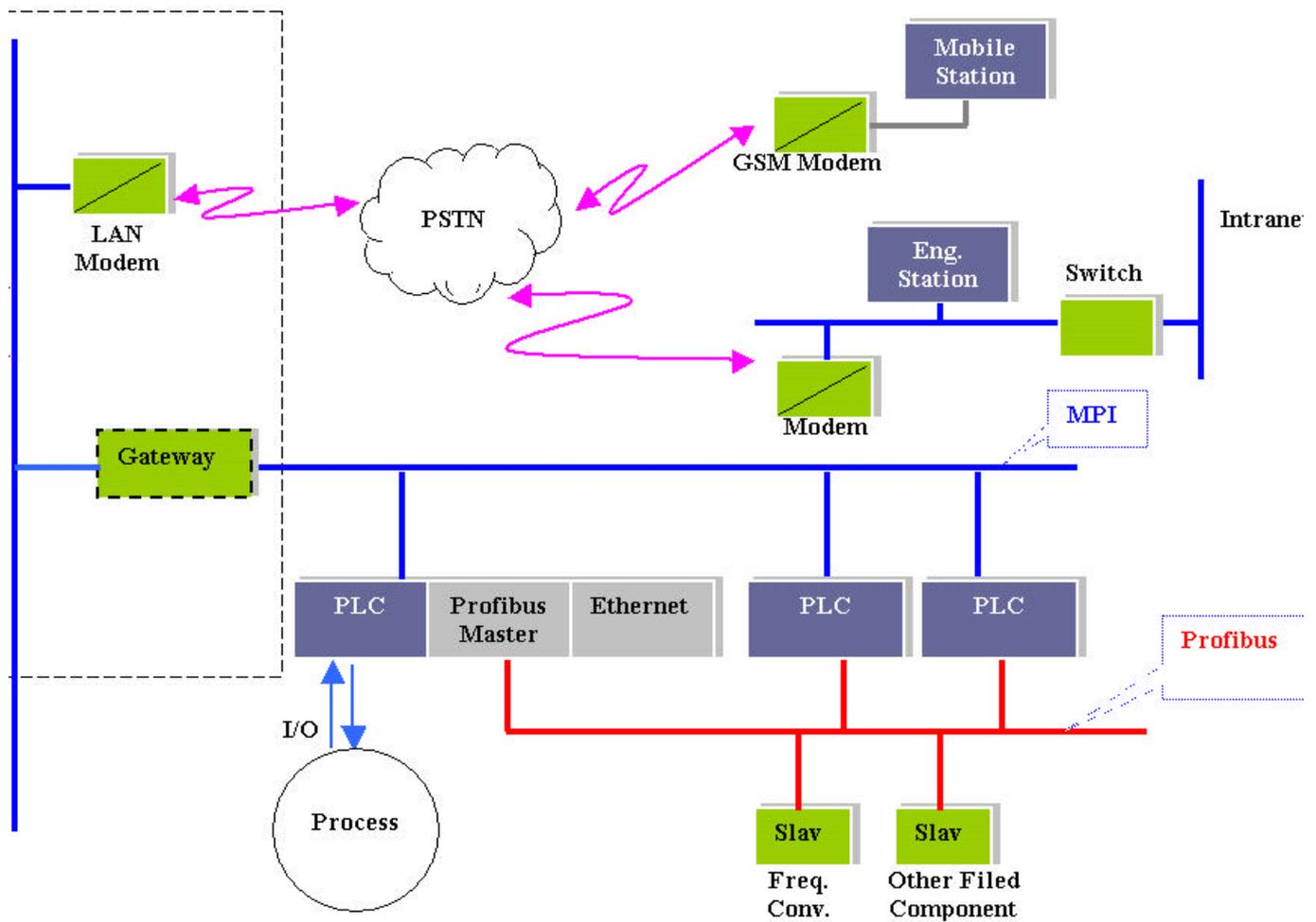
**Figure 5. The modem based solution**
