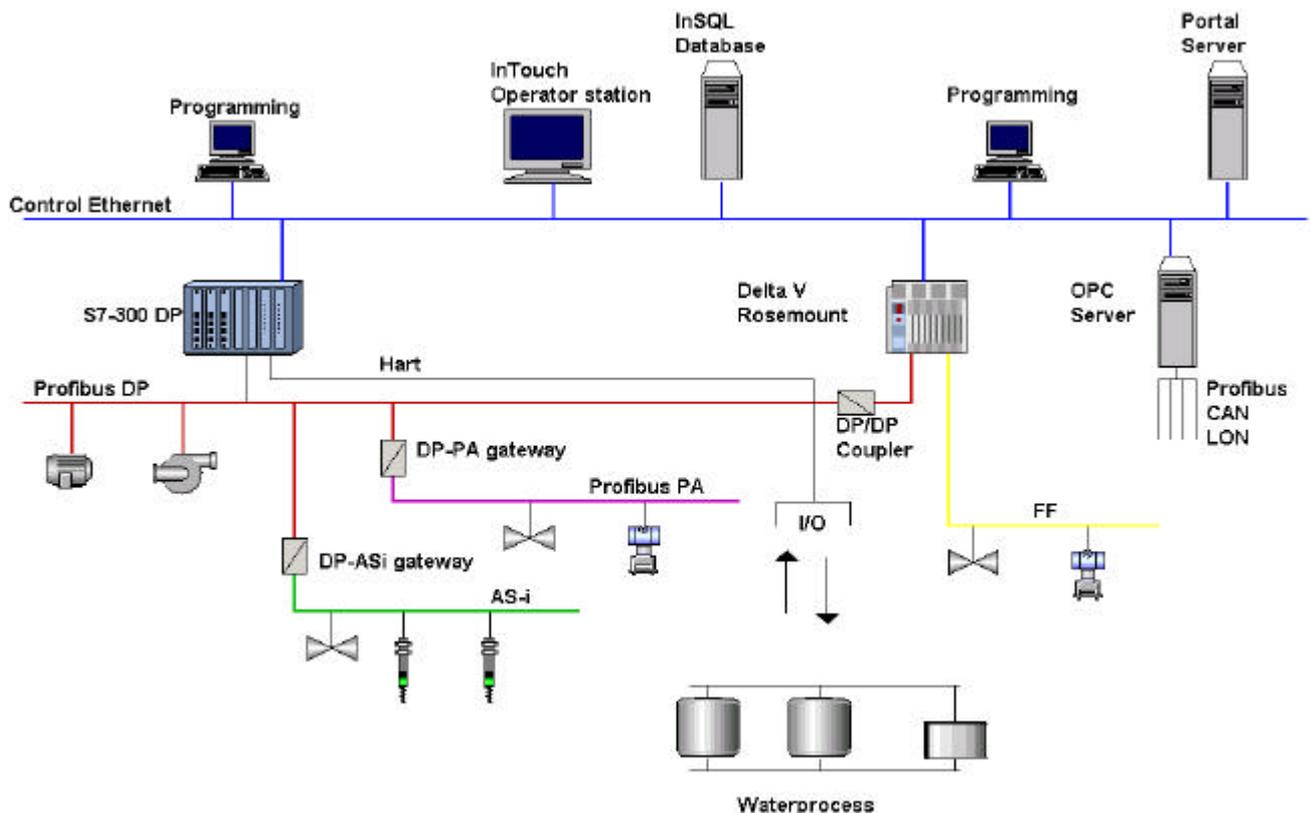
Figure 4. The system structure used in the Case Study
